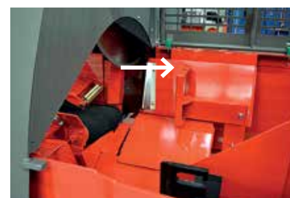
Adjustable splitting length from 250 mm up to 550 mm.
