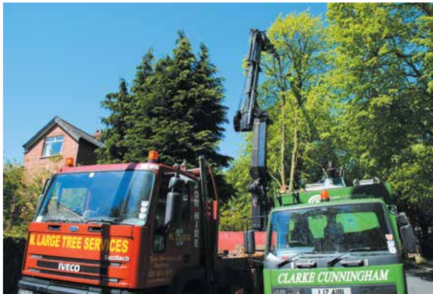
The Hiab XS700 E7 HI Pro mounted on an Iveco truck incorporates the latest control technology and safety systems. A 9-metre stabiliser span keeps the vehicle steady, even when the crane is working to the very limit of its reach and power.
