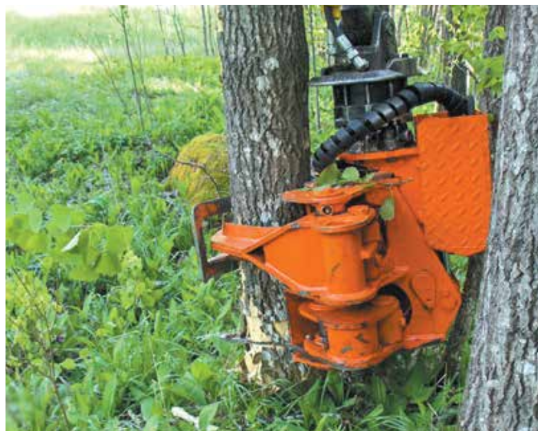
The Biojack energy wood grapple grabs a tree, cuts and delimits it before loading the log or stacking it at roadside.
