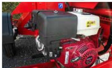
Powered by a 13 HP petrol engine.
