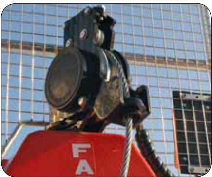
Device for wire rope unwinding (accessory) Available for models Farmi 60 – 85. Extend life span of wire rope and helps to unwind the wire rope to trees.
