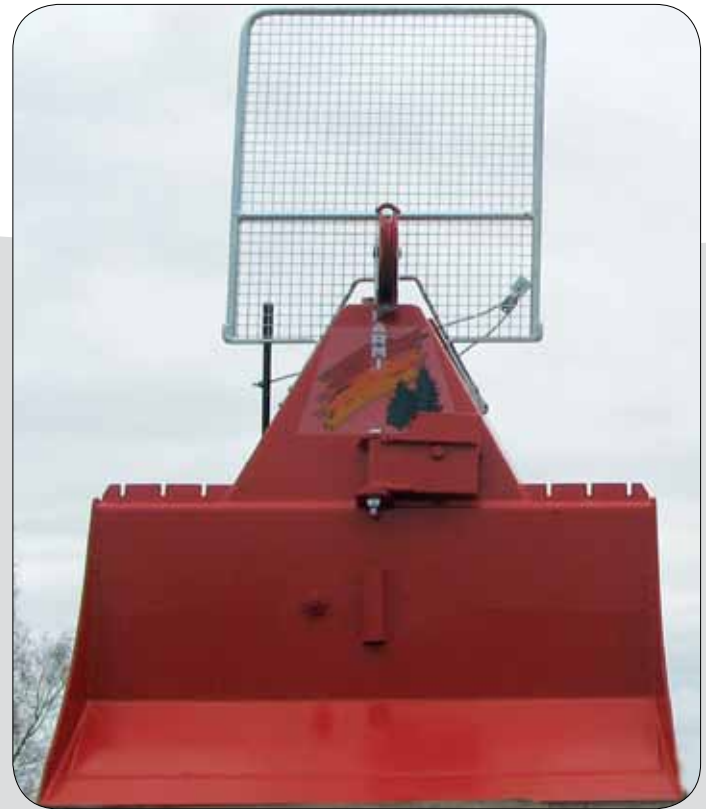
Farmi 60 with 60 kN line pull for tractors from 60 HP
