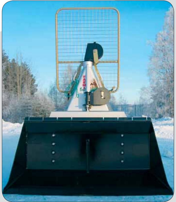
Farmi 85 with 85 kN line pull, high drum storage capacity and 2.0 m butt plate - excellently suited for professional applications with tractors starting from 85 HP.
