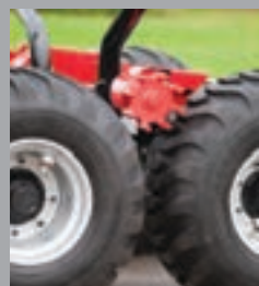
4WD - Farmiforest Vario 101 roll between tires operated four wheel drive
