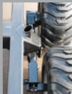
2WD - Sampo Hydraulics Blackbruin 2 wheel drive with hydraulic motors
