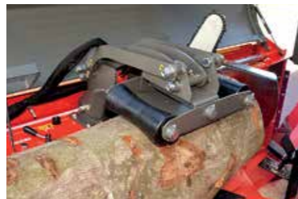
The hydraulic log press enables logs of all sizes to be sawed effortlessly.
