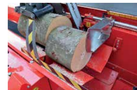
The guide plates ensure that even the shortest pieces of wood fall neatly into the splitting groove.
