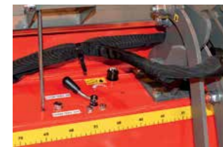
Automatic chain oil pump adjustment is easy to operate with the adjustment screw in the figure.
