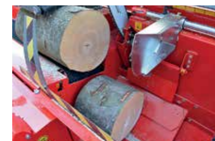
The guide plates ensure that even the shortest pieces of wood fall neatly into the splitting groove.
