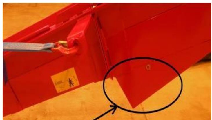
Belt tightness adjustment screw C (2 pcs/conveyor)
