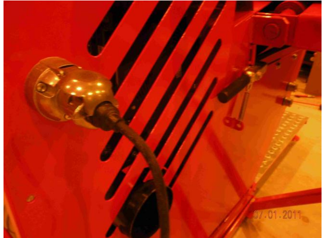
Figure 13. Connector of the optical measuring device
