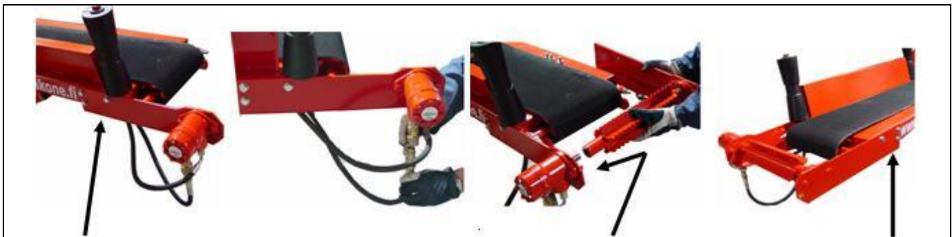
Figure 4. Installing the auxiliary input roller
