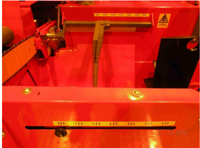
Figure 15. Log length adjustment
