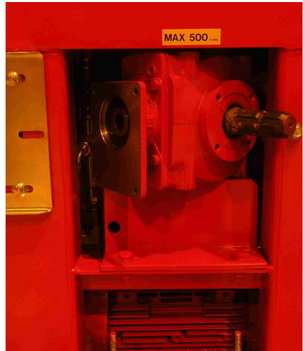
Figure 23. Replacing the angle transmission
