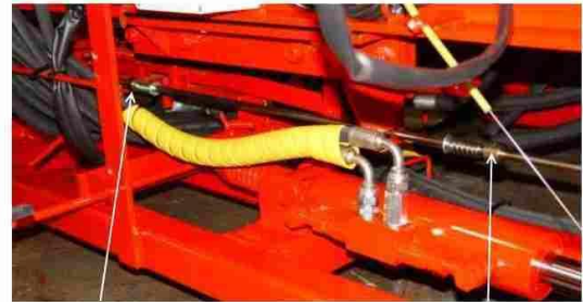
Figure 17. Cover plate for the stroke length adjustments
