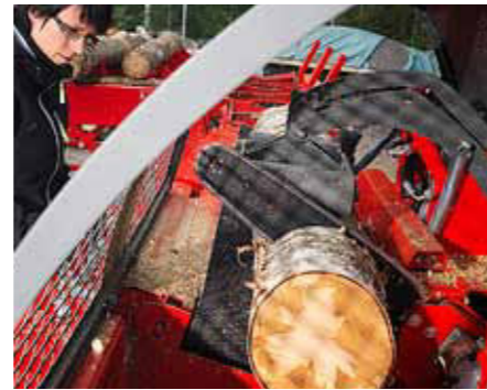
The wood is cut with a 20" hydraulic chain saw.
