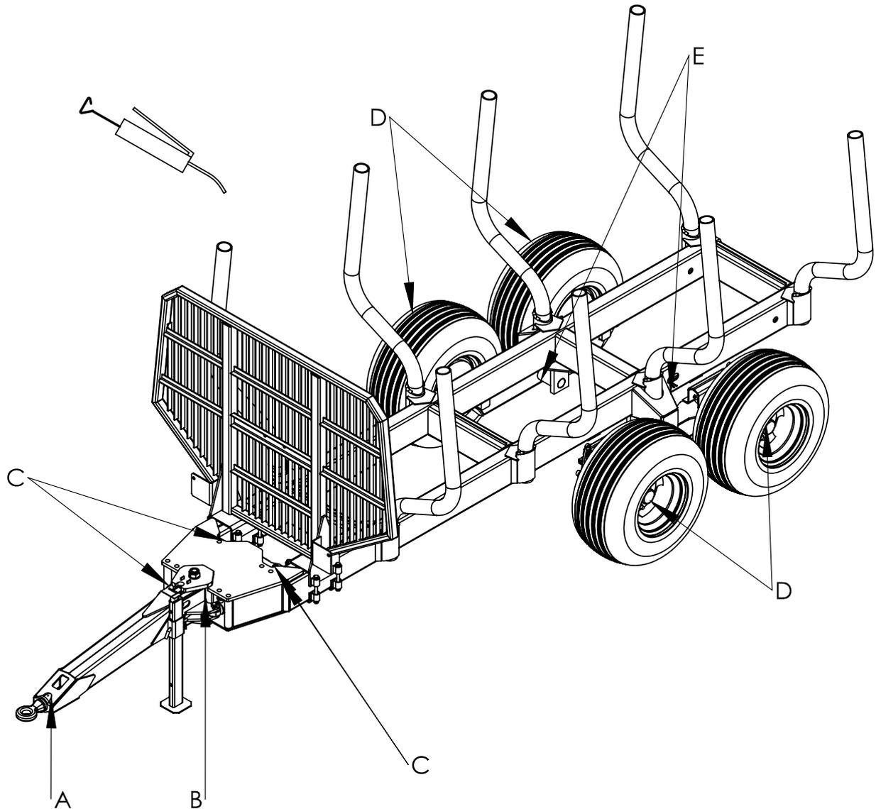
Figure 10. Lubrication points of Palms 10D forest trailer
