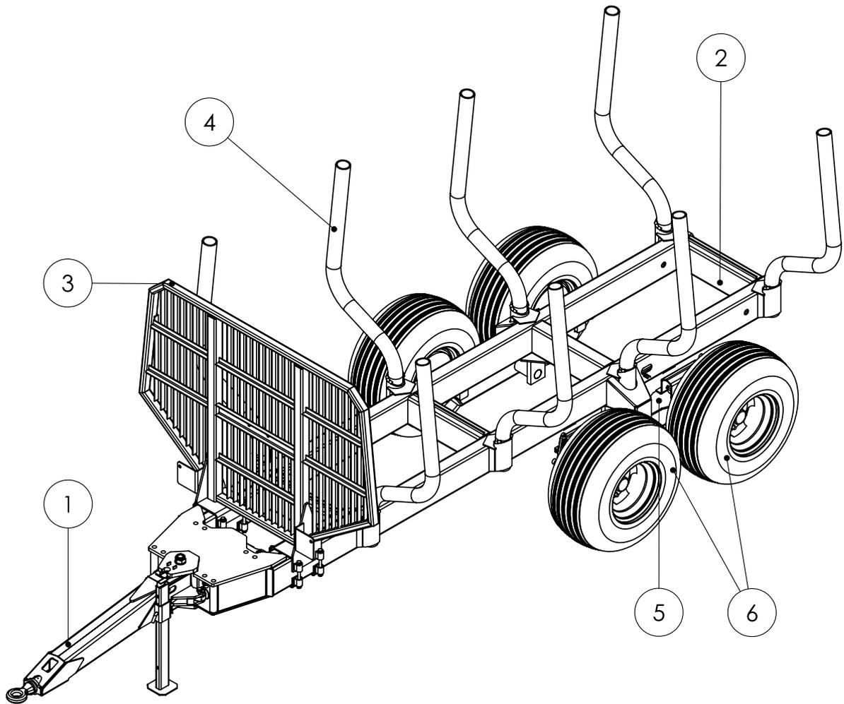
**Figure 1.** Basic components of Palms 10D forest trailer
