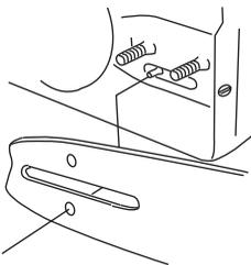
Tension the chain by turning the chain tensioning screw clockwise using the combination spanner. The chain should be tensioned until it does not sag from the underside of the bar. See instructions under the heading Tensioning the chain.
