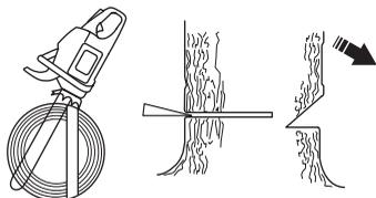
Finish the felling cut parallel with the directional cut line so that the distance between them is at least 1/10 of the trunk diameter. The uncut section of the trunk is called the felling hinge.
