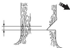
Set the spike bumper (if one is fitted) just behind the felling hinge. Use full throttle and advance the chain/bar slowly into the tree. Make sure the tree does not start to move in the opposite direction to your intended felling direction. Drive a wedge or breaking bar into the cut as soon as it is deep enough.
