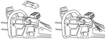
The filter can be cleaned more thoroughly by washing it in water and detergent.
