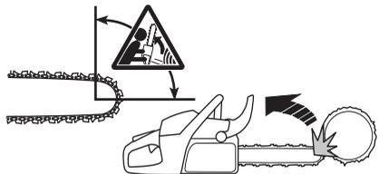
Cutting with the bottom edge of the bar, i.e. from the top of the object downwards, is known as cutting on the pull stroke. In this case the chain saw pulls itself towards the tree and the front edge of the chain saw body rests naturally on the trunk when cutting. Cutting
