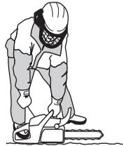
Push in the choke control as soon as the engine fires and keep pulling until the engine starts. When the engine starts, quickly apply full throttle; the throttle start lock will automatically disengage.
