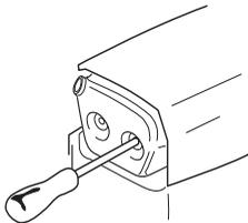
Some mufflers are equipped with a special spark arrester mesh. If your machine has this type of muffler, you should clean the mesh at least once a week. This is best done with a wire brush. A blocked mesh will cause the engine to overheat and may lead to serious damage.
