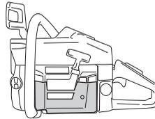
**CAUTION!** If the special winterising kit has been fitted or any measures have been taken to increase the temperature these changes must be reversed before the machine is used in normal temperature conditions. Otherwise there is a risk of overheating, resulting in severe damage to the engine.
