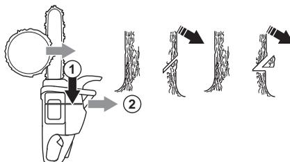
The directional cuts should run 1/4 of the diameter through the trunk and the angle between the top cut and bottom cut should be 45°.
